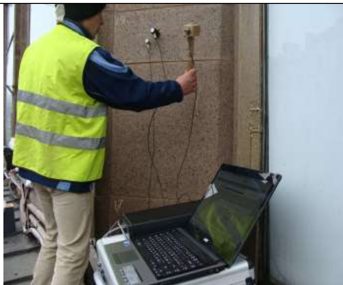
Fig. 2. Study of surfacing materials adhesion state using TKC-2 complex
